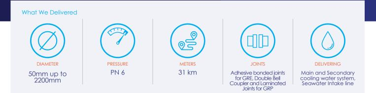
Wavistrong<sup>™</sup>/Alphacor Glass Reinforced Epoxy (GRE) pipe systems have high chemical and corrosion resistance as well as excellent mechanical, physical and thermal properties making them successful under the most demanding conditions. We supplied the project a range of diameters from 50mm up to 600mm.
