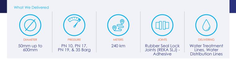
Future Pipe Industries supplied 240KM of Wavistrong<sup>™</sup> Glass Reinforced Epoxy (GRE) pipe with Rubber Seal Lock Joints and Adhesive jointing and supplied a total of 4,200 pieces of fittings.
