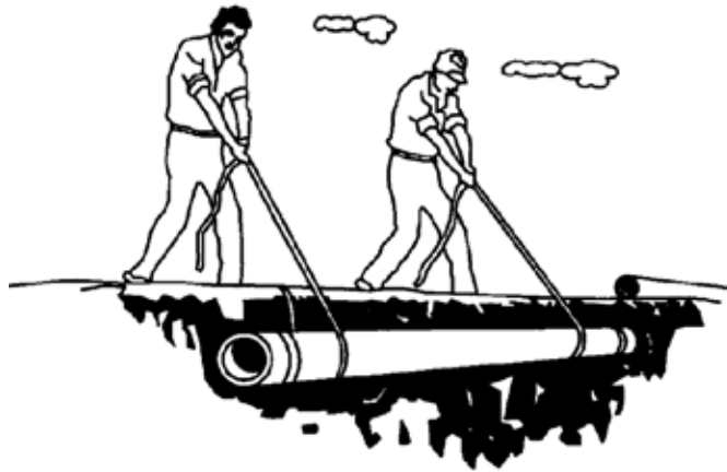
Figure 3: Lowering with ropes
