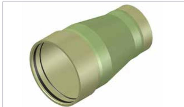
Concentric and Eccentric Reducers. Taper Length (L) =  $2.5 \times (D_L - D_S)$
