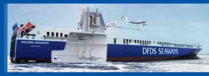
The International Maritime Organization (IMO) and US Coast Guard (USCG) put together in place a legislation for the cleaning of exhaust gases of ships. many ships need to be equipped with scrubber units to ensure cleaner air and a greener future.
