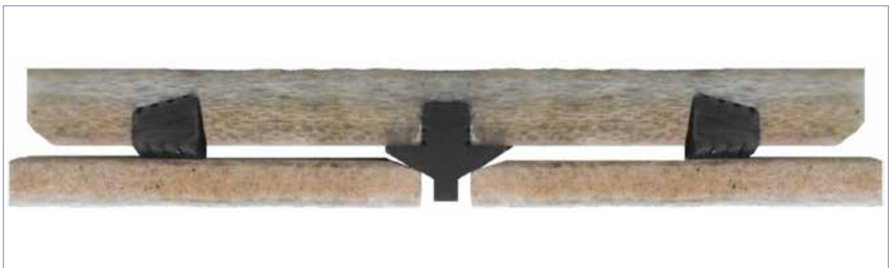
Figure 19.b - Double Bell Coupler with center register cross-section
