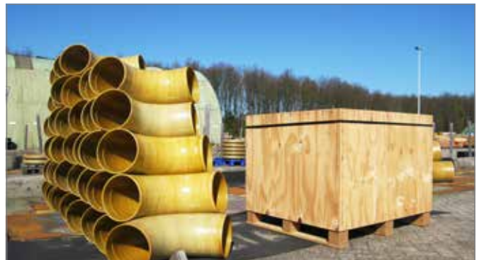
Fig. 3.11. Packing and storage of fittings
