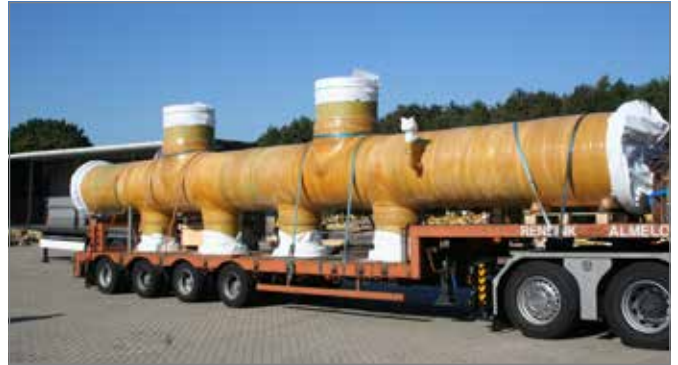
Fig. 3.5. Protected pipe/spool ends
