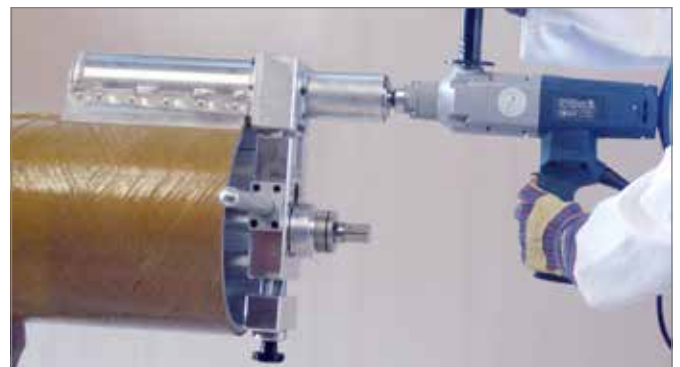
Fig. 5.2. Shaving of a spigot end
